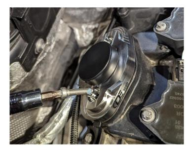
16. Now remove the alignment tool and insert the Dorch Engineering fuel pump. Use extreme **CAUTION** when installing the pump. The bolts MUST BE TIGHTENED EVENLY. Uneven loading of the spring can damage the pump. Also, be **EXTREMELY CLEAN** as all HPFPs are very sensitive to contaminants.
