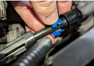
Once the collar is fully threaded on, use a wrench to tighten them. You may need to hold the hose in place by using an additional wrench on the hex portion of the hose fitting.
