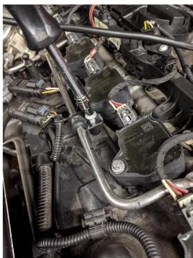
12. The high pressure line can now be completely removed, but **DO NOT SPILL** fuel on the coil pack boots.
