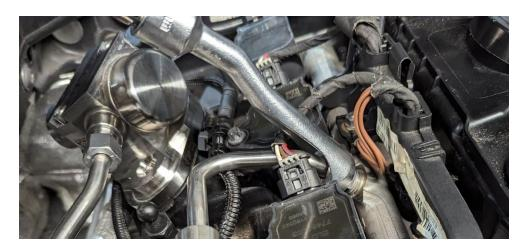
**NOTE:** We don't expect everyone to have specialty sockets for proper torque spec. In this case, simply "snug" the nuts with a 17mm wrench. 31nm is NOT a lot of torque so be sure to not over tighten and damage the line.
