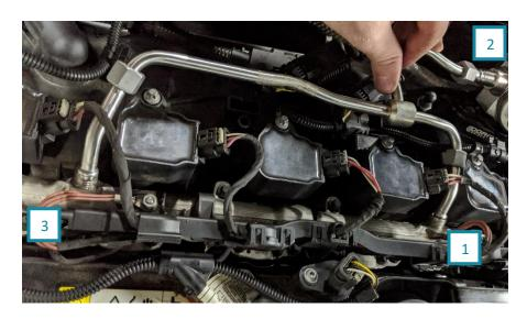
20. Lightly apply oil to the threads of the HPFP to prevent galling. If the nuts thread on effortlessly and bottom out with all the fittings well aligned, the three nuts can now be torqued.
