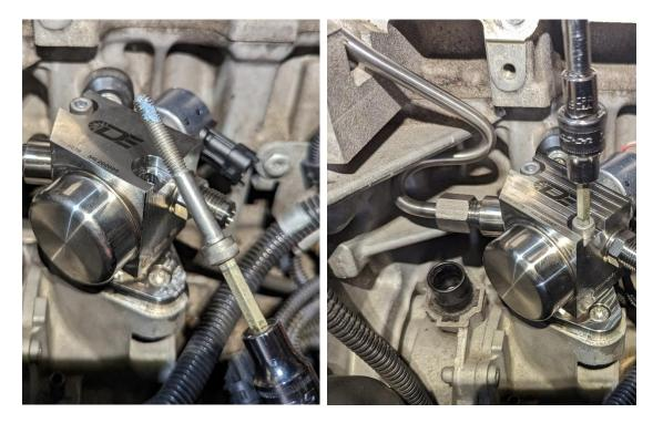
19. **READ THIS STEP THOROUGHLY.** Now connect the high pressure line to the HPFP. It will be a tight fit and the line **MUST BE AS STRAIGHT AS POSSIBLE** at the fittings.
