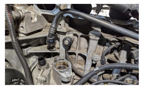
Knock Sensor Tightening Torque: 21.5nm
