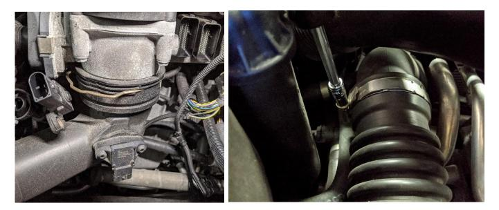
8. Next remove the four 10mm bolts holding on the throttle body along with the electrical connector and vacuum line:
