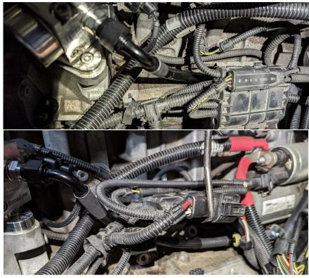
The male end of the Dorch hose will slide and click into the OEM hose. Once it's seated, pull back on the hose to ensure it's truly clicked in, then re-install the gray locking clip on the OEM hose.
