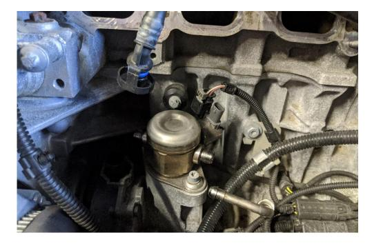
**<u>PWG Note:</u>** PWG cars will have an additional vacuum line to remove from the vacuum pump. This is a single line attached with a T25 bolt:
