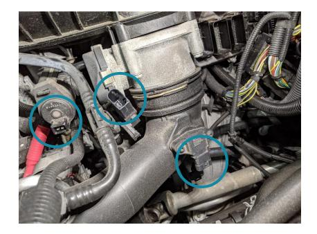
6. Remove the 2 vacuum connections pictured below and then unclip the line and purge valve from the intake manifold:
