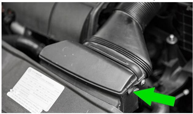
**3.** The air inlet is comprised of two parts, one section on the radiator support and another section of the air inlet on the engine cover. Separate these two halves by depressing the plastic tabs on both sides while lifting up on the engine cover side inlet section.
