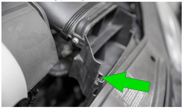
4. Unplug the mass air flow (MAF) sensor and place safely out of the way..
