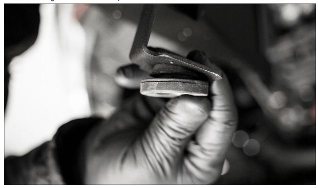
**16.** Install the velocity stack silicone coupler to the heat shield using 60mm-80mm hose clamp. Leave hose clamp loose in this step.
