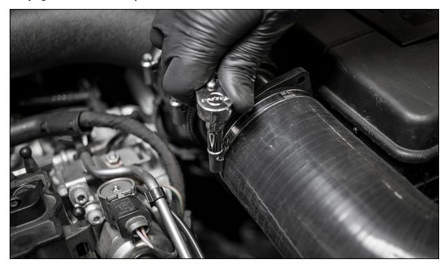
Install the air filter and included clamp onto the velocity stack.
