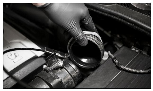
If your engine is equipped with secondary air injection, unclip and remove the SAI hose from the air box. Note: If you do not have SAI, skip this step.
