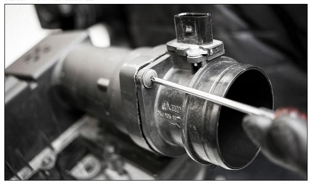
Remove the inlet pipe mount bolt from the bracket using an 8mm triple square.
