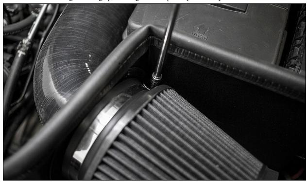
Verify all bolts, nuts, and harness clips are installed and tightened, all hose clamp connections are tight, and that your heat shield is fully installed. Start the car and inspect for any leaks or rubbing components. Enjoy the performance, looks, and sound of your new IE Cold Air Intake!
