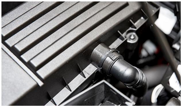
Remove Torx T25 bolt securing the back of the airbox. Pull straight up to remove airbox.
