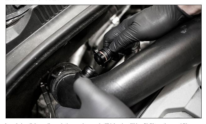
Loosely install the smallest reducing coupler onto the IE inlet pipe. Slide a 50-70mm clamp and 70-
