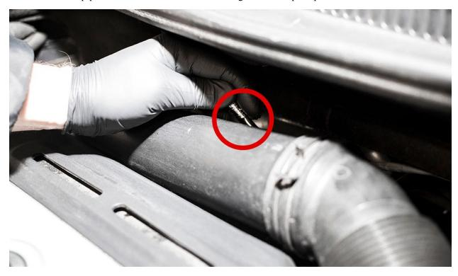
Using a hose clamp or pliers, loosen the lower clamp on the inlet pipe to turbo coupler. Pull the inlet pipe
