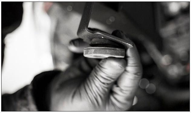
Line up the IE rubber grommets on the heat shield with the factory mount points.
