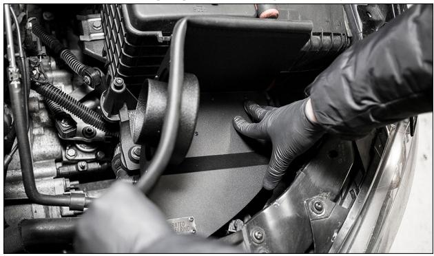
Install the straight reducing coupler onto the open end of the inlet pipe. Install 70-90mm clamps on both ends of this coupler. *Note: Do not tighten clamps in this step*.
