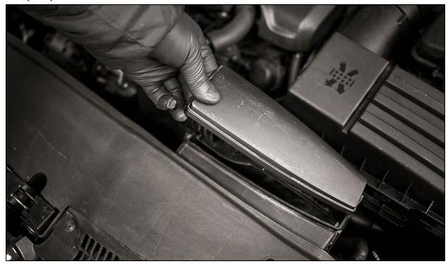
Remove the air duct from the car.
