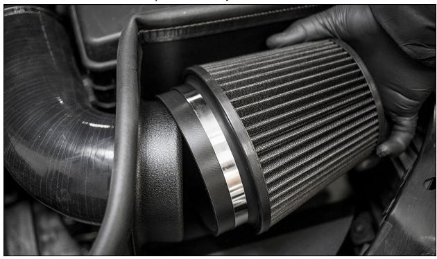
Rotate air filter so IE logo is facing upward. Tighten clamp firmly to velocity stack.
