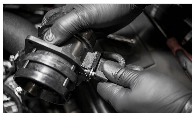
Slide MAF into coupler with the arrow facing backward. This is VERY important, as the car will not operate unless it is installed properly. We recommend installing the MAF with the wiring on the bottom side as a visual preference.
