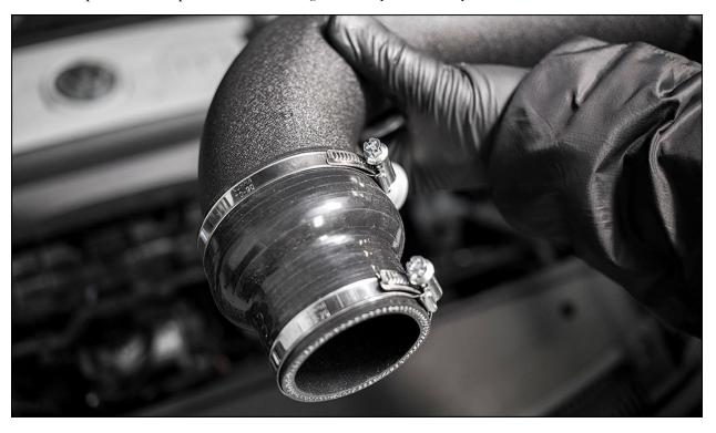
Push coupler onto the inlet of the turbocharger, confirming that the coupler is on entirely. Tighten lower hose clamp only with a 7mm socket.
