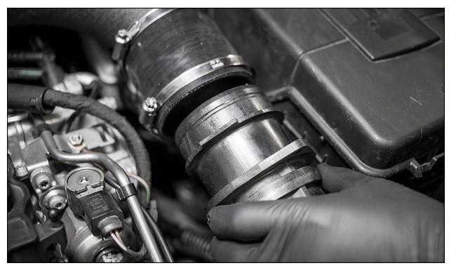
Install large elbow coupler and 80-100mm clamp between velocity stack and MAF.
