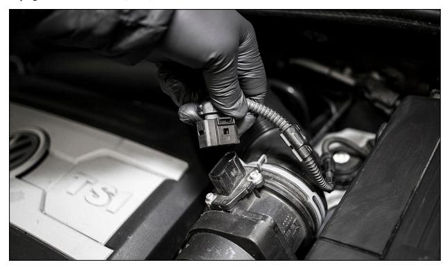
Using a hose clamp tool or pliers, remove the spring clip that holds the inlet pipe to the MAF. The clamp can be moved onto the pipe behind the MAF. Remove hose from MAF.
