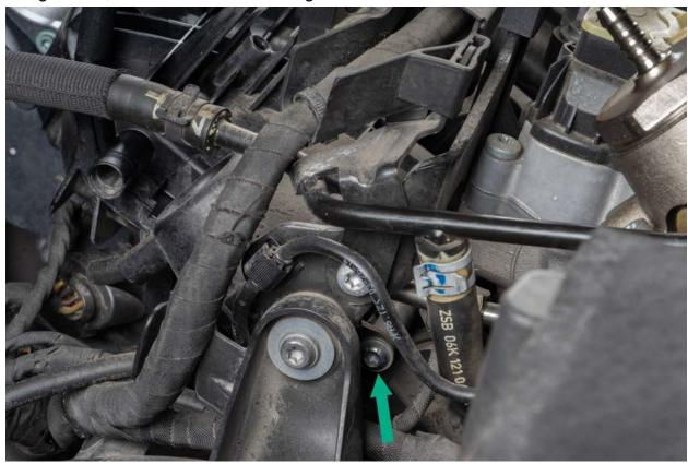
Using number 10 Triple square, remove the HPFP Bolts from the top of the pump
