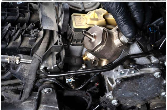
Remove the pump from the housing.
