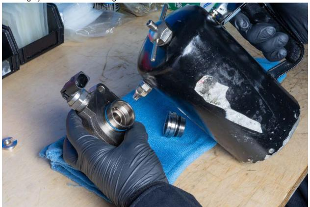
Lay out all the new IE components, pump body, and the stock spring in your clean environment. Inspect and clean all parts of any contaminants (dust, dirt, lint, etc.)
