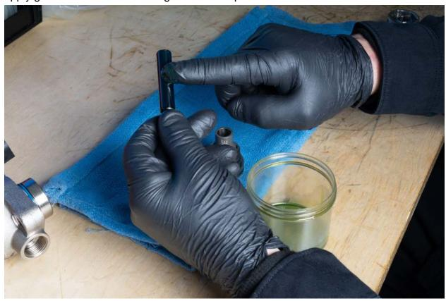
Insert pin small end first through the small side of the cylinder. Push until the tip of the pin has clearance to insert the retainer. **NEVER** install the opposite direction or seal damage will occur.
