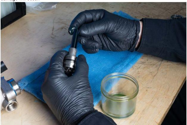
Install factory spring over the pin seated on the assembly body.
