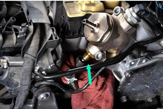
Using T30 bit, remove the screw holding the fuel line bracket
