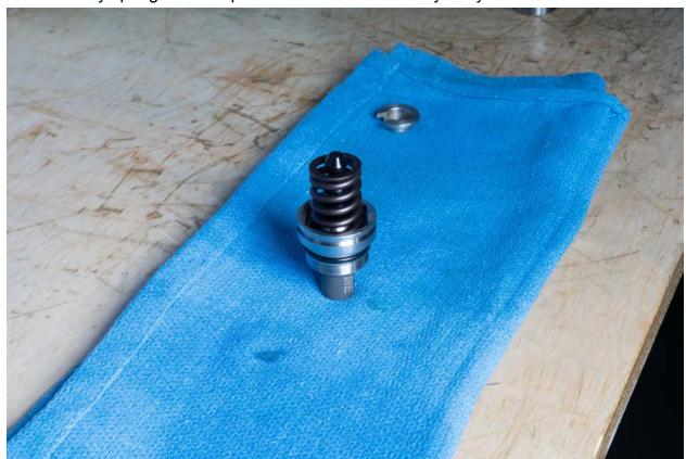
Line up the notch on the retainer with the groove on the pin and press down on the spring to install the retainer. Bottom of retainer should sit flush on the spring.
