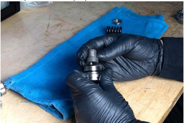
Apply generous coat of clean engine oil to the pin.
