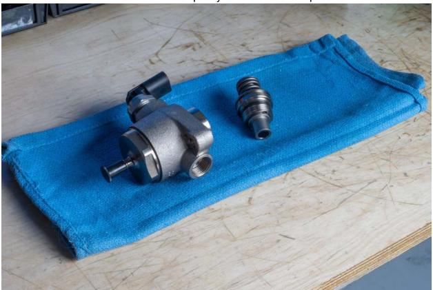
Using a hydraulic press, line up a similar-sized bit to the stock HPFP pin and press it out of the retainer to release the spring. Remove the stock spring and set aside for re-assembly with IE parts.
