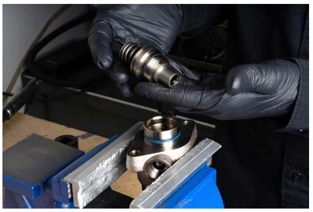
Prepare an incredibly clean surface, this is *very* important as any contamination can cause issues with seals or wear on the pin/cylinder and lead to premature failure.
