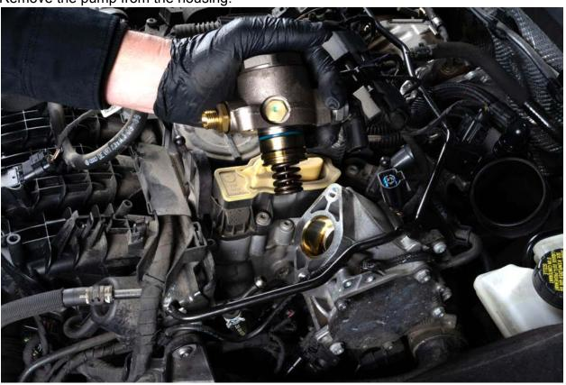
Pull the HPFP internal assembly from the pump using your IE assembly tool (part number IEFUVN1-4), ½" drive socket wrench, and a bench vise.
