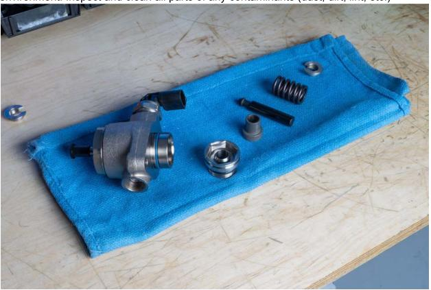
Install the cylinder into the assembly body as shown below.
