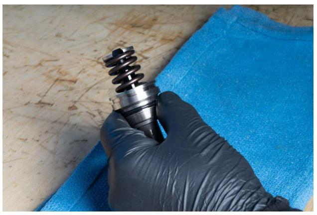
Hand thread the complete IE internal assembly into the HPFP pump. Using IE HPFP assembly tool, torque the internal assembly to 45ft-lb.
