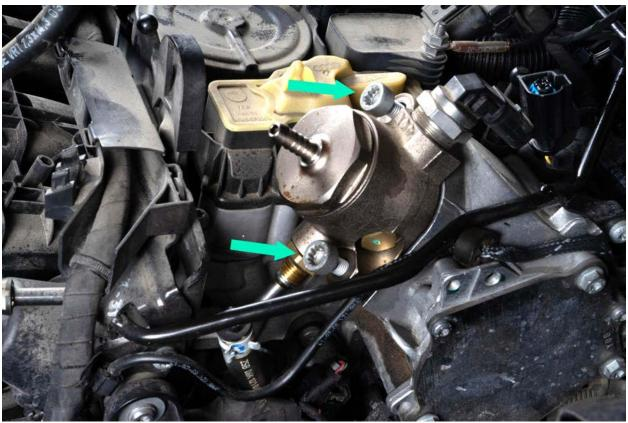
Factory procedure says that this lower supply line nut pictured should be removed, however you can save lots of time by gently pressing down on the high pressure fuel line while twisting the HPFP to the drivers side. This will help the fuel line clear the fitting. Take caution to not bend, deform or crush the line. Simply apply enough pressure to allow the line to clear the fitting.
