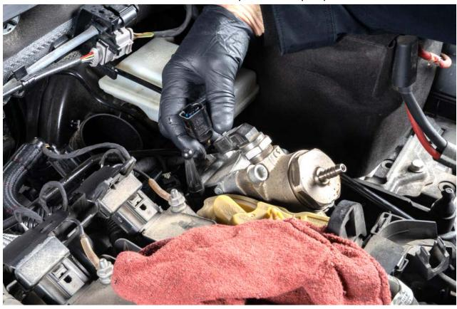
Place a rag around the high pressure fuel supply line and using a box end wrench, loosen the nut, then place the rag below and remove the nut from the supply line.
