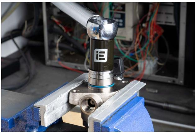
Install the HPFP back into the vehicle in reverse order. Once all fittings and lines have been attached and tightened, start the vehicle to verify there are no fuel leaks. Congratulations, your HPFP is now upgraded.
