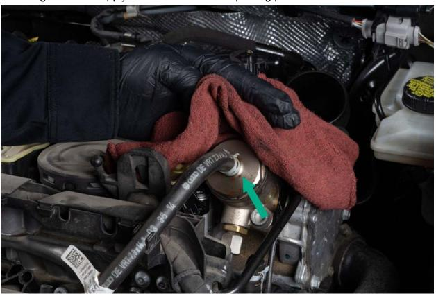
Remove Fuel Supply Line from Fuel Pump
