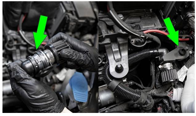
Line up the IE intake heat shield or intake box push grommets with the posts and reinstall intake. This will securely sandwich the the SAI filter bracket and cleanly tuck and hide your SAI filter under the heat shield/intake box.
