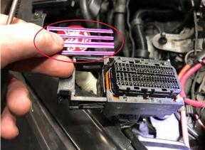
47. The connector has plastic blanks to fill in the holes where there are no terminals inserted. Note how the connector is numbered in the first photo. Using an electrical depin tool or paperclip remove the plastic blanks from the locations shown in the second photo. (reference step 49 for pins to remove)
