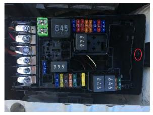
57. Reinstall the front cover by sliding it down into place until it locks. Then install the factory box cover.
