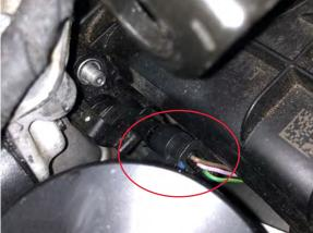
19. Unplug the connector for the second map sensor located on the top of the intake manifold then pull the fuel line up from the tabs located on top of the manifold.
