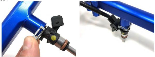
33. Lubricate the remaining O-ring on each of the 4 injectors and align the injectors with the holes in manifold as seen in the first photo. Then firmly push the fuel rail until the fuel rail is fully seated against the intake manifold. Install the two supplied bolts, for cars that came equipped with MPI install rail using original hardware from the factory plastic fuel rail.
