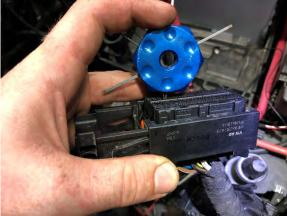
48. While removing the terminal blanks from the 105 pin connector you noticed they each face a certain direction this locks them in place in the connector when the purple locking slide in installed.
