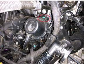
43. Route the provided wire harness along the same path of the factory harness down the driver side of the engine. Continue routing the wiring along this path until it reaches the ECU. Secure the wire as you go with tie wraps.
