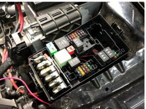
53. Remove the front cover of the fuse box by grasping the cover and pulling up to slide the cover off while releasing the locking tab.
