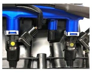
34. Remove the supplied harness from packaging and start at the opposite end of the Red wire. The two connectors (male female) connect to the factory intake runner flap position sensor. Connect the factory runner flap connector to the supplied harness and then plug the matching connector on the new harness into the runner flap position sensor.
