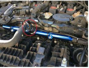
38. Reinstall the 10mm triple square bolt and 13mm nut to the support brace under the manifold. Tighten both hand tight first. Then once both are installed torque the 13mm nut followed by the 10mm triple square bolt.
