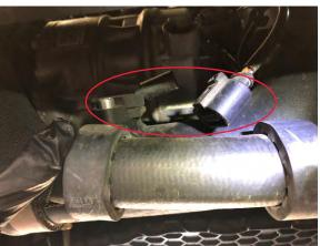
10. Remove the remaining T30 screw securing the throttle body inlet pipe. Disconnect the throttle body inlet pipe from the throttle body and let it hang down.
