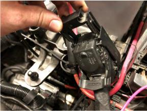
52. Remove the top cover from the fuse box. Then pull the tab at the front of the fuse box and lift the slide door as shown in the photos below.
