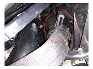
8. Locate and remove the two T30 screws used to secure the throttle body inlet pipe and turbo outlet pipe to the block. Unclip the harness connected to the turbo outlet pipe at this time.
