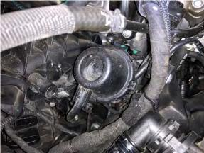
13. Remove the remaining T30 screw securing the turbo outlet pipe to the engine, then disconnect the turbo outlet pipe from the turbo and intercooler by losing the hose clamps as needed. Then Remove the turbo outlet pipe from the car.
