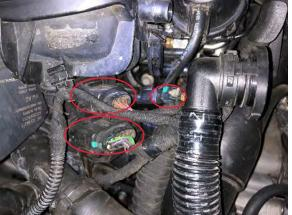
42. Reconnect the Cam position sensor on the driver side of the intake manifold as shown below.
