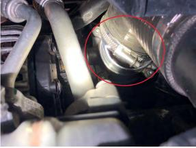
11. Disconnect the three electrical connectors located on the driver's side of the intake manifold.
