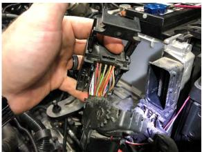
46. Using a pick tool or small screwdriver remove the purple locking tab by sliding it from inside the connector.
