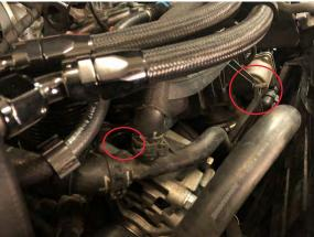
4. Remove the intake using instructions from the manufacturer of your intake kit if needed.
