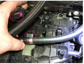
20. Remove the two 10mm nuts from the passenger side of the intake manifold. Then remove the eight T30 bolts securing the intake manifold to the cylinder head.
