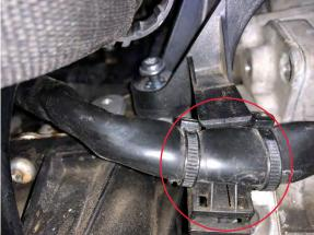
9. Unclip the harness connected to the turbo outlet pipe, and then disconnect the connector for the MAP sensor located on the throttle body inlet pipe.
