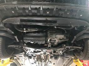
7. Locate the lower radiator hose and disconnect the plastic clamp securing it to the front of the engine.
