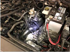
5. Disconnect both the cold side charge pipe & electrical connector from the throttle body.
