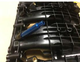
28. Tighten the supplied 7mm drill bit where just the end of the bit is in the chuck of the drill (the bit is just long enough to go through the port). Then drill through the center of the injector port prep tool using high speed on the drill bit and minimal force until the bit passes through the inside of the intake manifold. Repeat steps 24 & 25 for the remaining 3 holes.
