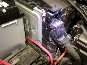
45. Ensure the lever on the connector is fully open. Then use a small screw driver to pry the cover and lever off the 105 pin connector as shown in the photos below.
