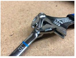
25. Place the threaded brass insert over the top of the hole and by hand without any tools start screwing the insert into the manifold making sure the insert is straight in all directions. Then once the insert is straight in all directions heat the outside of the manifold in the area the insert is being installed with a heat gun. Be careful not to overheat the plastic you want it hot enough that you can hold your finger to it for a couple seconds before you need to pull your finger away.
