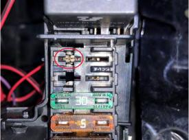
56. Reinstall the fuse panel into the fuse box pushing aligning each of the T shape alignment tabs on the box with the fuse panel. The panel should lock back in place just as it was previously. Install a 20amp fuse in this new fuse location.
