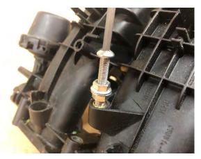
27. Secure the supplied injector port prep tool into a drill firmly so that it cannot spin inside the drill chuck. With the drill in clockwise rotation drill down into the injector port until the tool stops going down. Stop drilling and without removing the tool from the manifold disconnect the drill from the injector prep tool.
