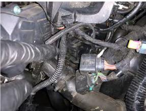
12. Disconnect the Intake manifold runner flap control valve and camshaft position sensor connectors located on the driver's side of the intake manifold & cylinder head.
