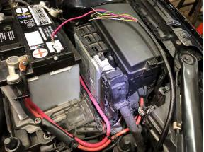
44. Disconnect the 105 pin connector form the ECU located next to the battery and fuse panel by flipping the lever on the back side of the connector down while lifting up on the tab on top of the connector.
