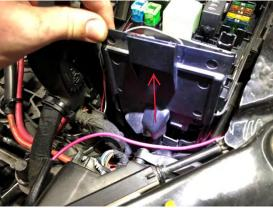
54. Using your hands through the back portion of the fuse box pull up while releasing each of the clips securing the fuse panel to the inside of the fuse box. This step requires a decent amount of force take your time and ensure each securing clip is released as you pull.
