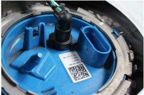
7. Once the car stalls out it is time to disconnect the fuel line. The line will still have a decent amount of pressure use a fresh rag to cover the assembly and soak up any fuel. Quick connects always work best by pushing down first on the connector then pushing in on the release and pulling up. Pull up slowly as full will spray out and have it covered with a rag to not make a mess. Allow the remaining fuel to soak into the rag so that it can be discarded.
