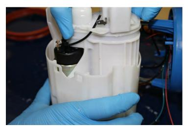
15. With the pump removed from the bucket, take a razor and clean any remaining plastic flashing from the holes. This is also a good time to remove any plastic or dirt from the bucket (we recommend compressed air for this).
