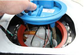
9. **DO NOT LIFT THE ASSEMBLY OUT OF THE TANK AT THIS TIME** as damage can be caused by the fuel float being caught on the inside of the tank! Disconnect the fuel float from the sending unit by using a small screw driver or pick tool and popping it up from the lock then remove the float from the tank first.
