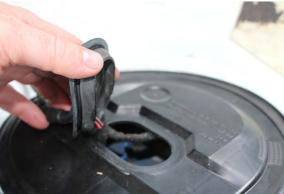
4. Remove the plastic cover by pushing the cover towards the rear of the car firmly and pulling up on the front. Careful not to break the plastic tabs from the cover.
