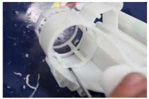
21. Mark the plastic as shown in the image below and carefully cut using a rotary tool, sharp razor, or other cutting tool of your preference.
