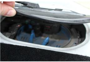
5. Using a flat blade screwdriver pull up the red locking tab (it does not require much pressure). Then disconnect the electrical harness from the fuel pump.
