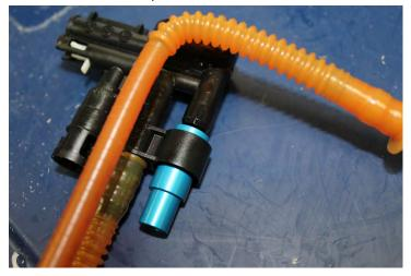
18. Remove the fuel filter from the bottom of the pump using a flat blade screwdriver.
