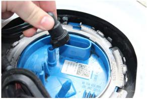
8. Using a large flat blade screw driver and hammer if needed tap the lock ring in a counter clockwise rotation until the ring is released. Remove the ring and the pump should be released (it will pull up easily as shown).
