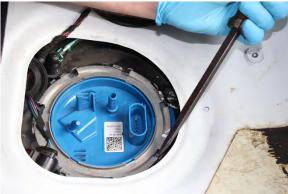
31. Connect the electrical connector and fuel line as shown below and start the car. It might take 2 or more attempts to start the car as we have removed fuel from the lines during this process. Let the car idle for 1-2 minutes then rev the engine lightly. Once you have ensured the motor runs smooth like before and there are no lights on the dash related to fuel pump you can install the plastic dust cover and set over the pump and assembly is complete.
