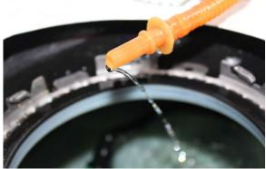
11. With the pump assembly removed from the car push down on the top hat and remove the lock ring from the shaft with spring as illustrated below.
