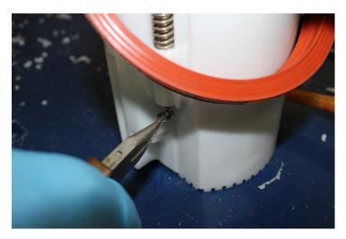
12. Now remove the sending unit from the bucket by pushing the two release tabs near the top of sending unit and pulling up. (the two release tabs release the catches shown in the second photo)
