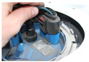
6. With the harness now disconnected from the fuel pump start the car, we are now depressurizing the fuel line it can take a couple minutes for the car to stall out. Ignore any dash lights resulting from the plug to the pump being disconnected. While the car is idling use this time to push the rubber grommet through the dust cover and take a rag and clean the top of the fuel pump assembly.
