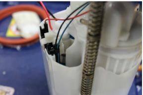
24. Once you have verified fitment of the sending unit, remove the sending unit as shown in step 12 of this manual then remove the assembly from bucket. With the assembly removed insert the pump mount locking ring as shown below and insert the pump into the assembly installing the fuel filter as keyed to the pump.
