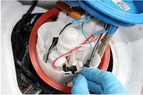
30. Seat the pump fully into the tank ensuring the alignment tab is in the correct position. Then proceed to install the locking ring into place using a large screw driver and hammer if necessary to turn the ring until the ring is tight. (Tip: Moving the screwdriver to different locations on the ring and tapping works best to seat it)
