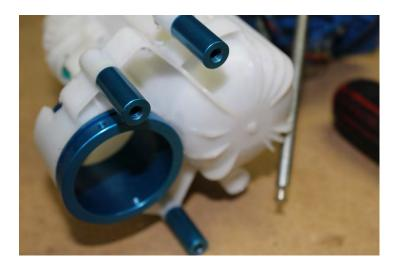
23. Re install the sending unit as shown and ensure that it clicks in place with little to no force. If it does not then the sending unit is hitting somewhere and more trimming needs to be done. Remove the assembly from the bucket and trim as needed to gain clearance. Also ensure the sending unit arm can move freely from side to side without making any contact with anything.
