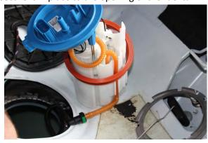
29. Insert the pump into the tank rotating counter clockwise until the electrical connection on the pump assembly is located parallel to the back of the car. Then reinstall the fuel float as it was removed in step 9 of this install guide.
