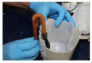
17. With the venturi removed from the bucket you can now install the venturi extension seen in the photo below.
