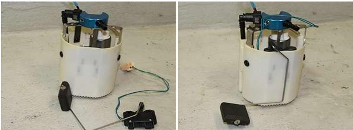
25. Locate the two alignment tabs located on the top hat that were previously needed with the factory design. Using a cutting tool cut these tabs off close to the base. It is not required to be flush however they need to be removed within 1/8" - 1/4" from their base.
