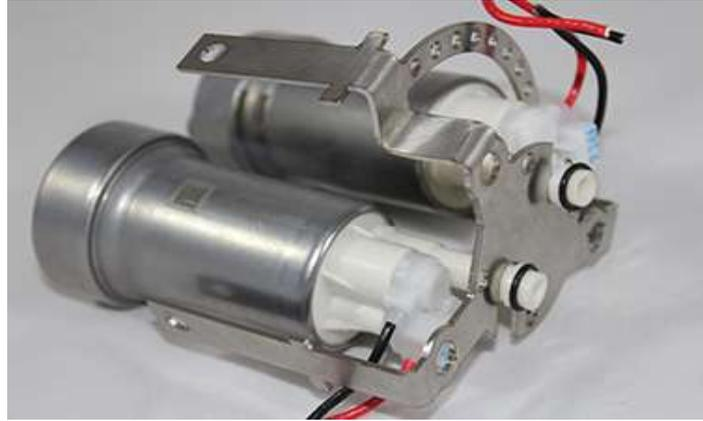
9. Install 3 of the 4 screws as shown below (2 on side with venturi tighten down), on the other side install 1 screw only a turn or so. Slide the pump support under the loose screw and install the 4<sup>th</sup> screw once lined up. Continue to tighten all 4 screws until they are tight while holding the pumps.
