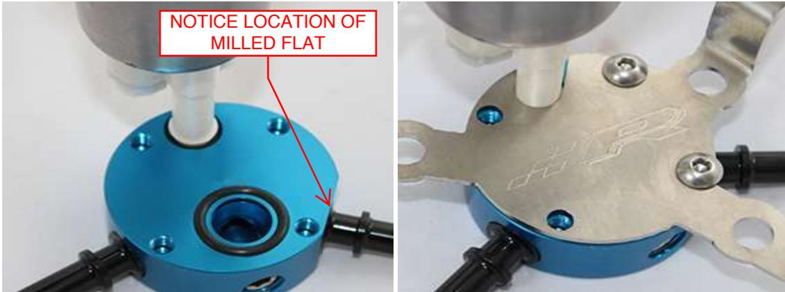
18. The pump will now be supported by the bracket but it needs to be treated with care for now. Install the 3<sup>rd</sup> screw as shown by only screwing in a couple threads. Once it is in slide the pump support bracket under the screw and install the 4<sup>th</sup> screw. Complete tightening of all 4 screws using a 3mm allen wrench.
