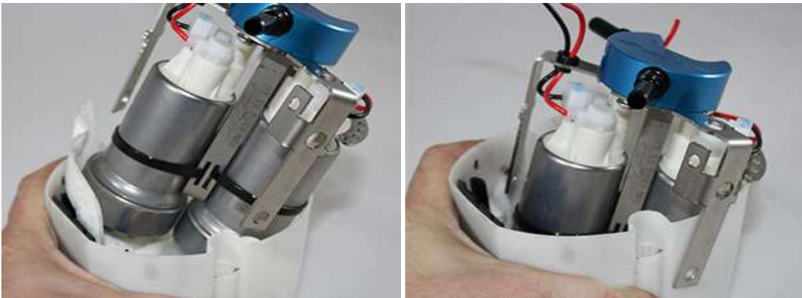
13. Once the assembly is in with all 3 legs inside the bucket you can reconnect the venture line and reinstall the 3 nylon push rivets.
