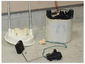
4. Carefully locate and pry loose each of the 3 points, the black upper piece is secured to the white bucket. Heat can be applied but ensure there are no remains of gas or gas fumes. The best tool for the job is a small screwdriver and pick tools. The plastic can crack and minimal damage is ok and will not affect functionality but taking your time will ensure no damage to the bucket itself.
