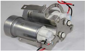
Install 3 of the 4 screws as shown below (2 on side with venturi tighten down), on the other side install 1 screw only a turn or so. Slide the pump support under the loose screw and install the 4<sup>th</sup> screw once lined up. Continue to tighten all 4 screws until they are tight while holding the pumps.
