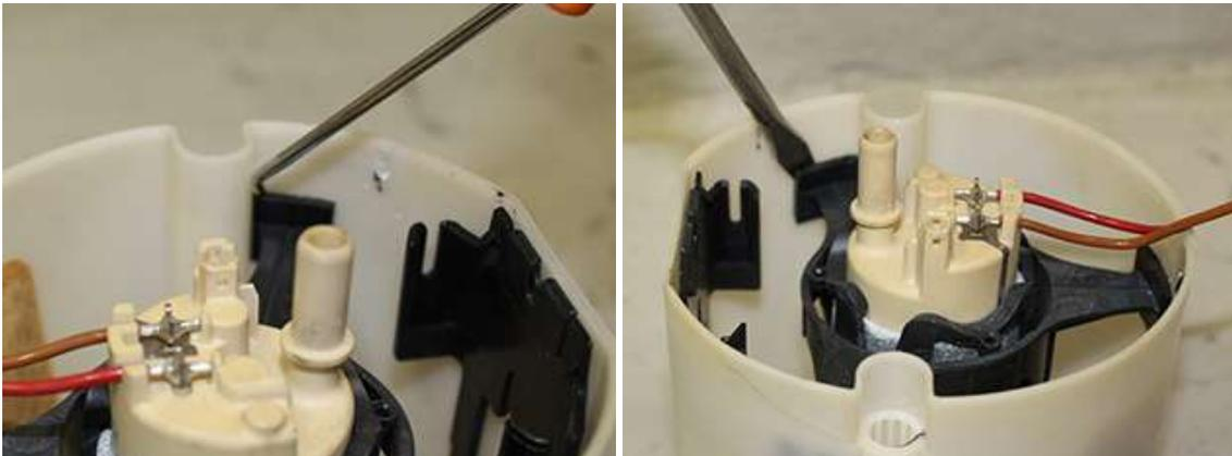
6. Next step is to remove the fuel sock and venture from the bottom of the pump. For this you simply take a screw driver as shown below and pry up on the fuel sock. Once the fuel sock is removed take your screwdriver and carefully push the venturi out as it is simply pushed into a hole on the fuel pump.
