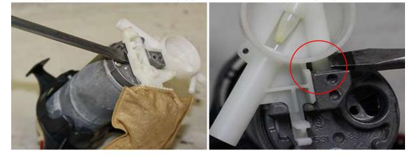
7. The next step is to cut the factory wiring going to the fuel pump. There is plenty of wire but it is always good to make sure you have plenty so cut about where shown in the image below. Once the harness is cut keep the connector end we will be reusing it. Take the other 3 items below and place them aside we will not be reusing them in the assembly of your Stage 2+ kit.
