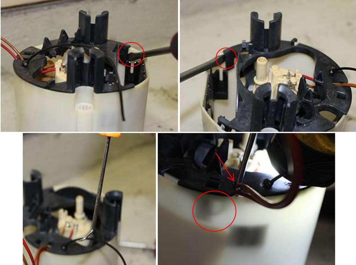
5. As done in the previous step you have 3 more points where the stock fuel pump was glued together. To remove these as before use a pick tool to gently work the tabs loose of the bucket. Once you get clearance enough to slide your screwdriver in it can be pushed in the slot like a wedge and wiggled back and forth. After all three glued joints are loose remove the fuel pump from and mount from the bucket by lifting up.
