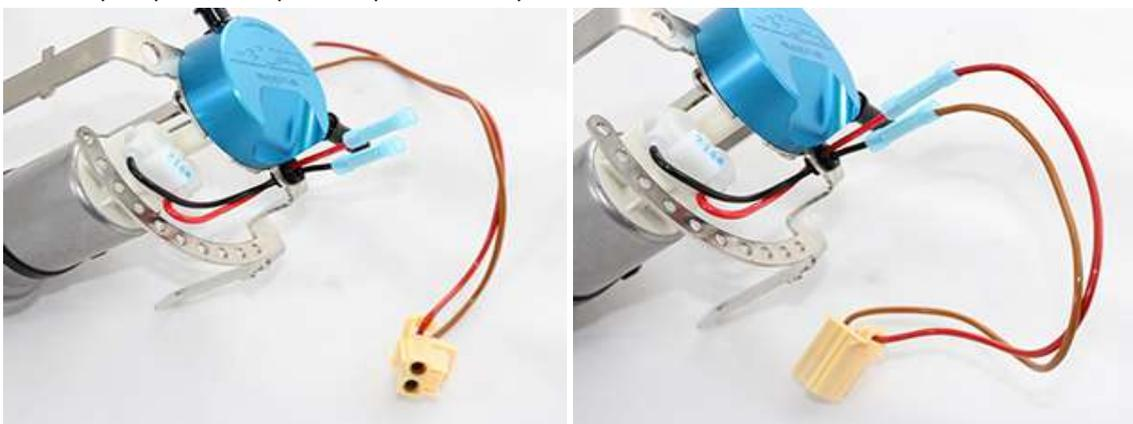
22. Insert the remaining 2 nylon zip ties supplied in your fuel kit as shown in the image below, do not tighten them completely only a few clicks are required for this step. We are preparing for future use during installation.
