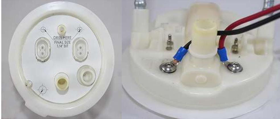
16. Install the pump and reconnect the return lines as shown in step 28 of the Stage 2+ assembly instructions. Connect the 2 mating wire spades previously installed for the Stage 3+ fuel pump. Install top hat and secure the lock ring with the tools provided in your Stage 2+ kit.
