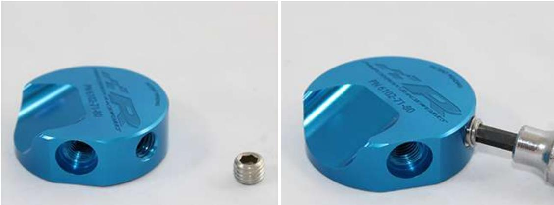
14. Take the blue manifold with the stainless plug inserted and two fittings supplied in your Precision Raceworks Stage 2+ Fuel Kit. Screw both fittings into the other two holes on the OD of the part. The fittings come with O-ring seals preinstalled. Once the O-ring makes contact with the hole in the manifold they might need some pushing inward to continue going into the fitting.
