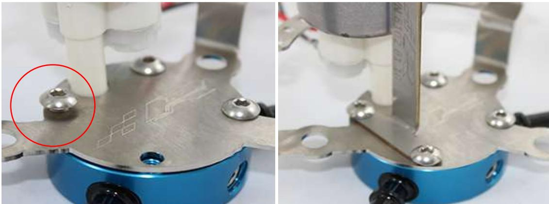
19. Secure the pump to the support using the supplied nylon zip tie being sure to keep the lock portion of the zip tie close to the stainless steel support as shown below. Once it is tight cut the excess off as shown.
