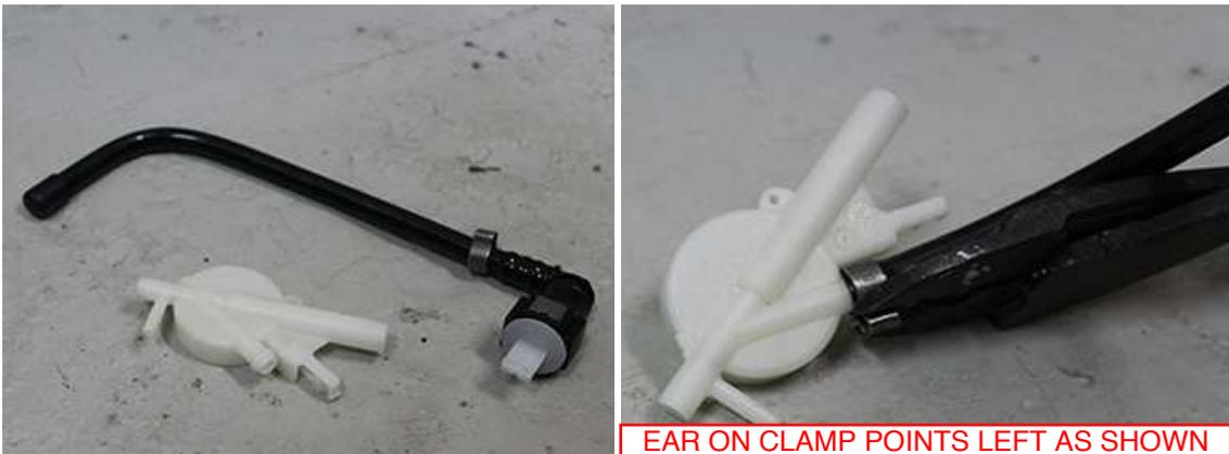
11. To install the venturi drill 4 holes using your small drill bit and working up to one large enough for the supplied nylon zip ties to pass through the holes. The holes do not have to be on an EXACT location but the images below and use of a flashlight can help better understand where to drill the holes.
