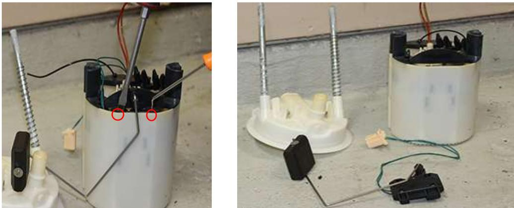
4. Carefully locate and pry loose each of the 3 points, the black upper piece is secured to the white bucket. Heat can be applied but ensure there are no remains of gas or gas fumes. The best tool for the job is a small screwdriver and pick tools. The plastic can crack and minimal damage is ok and will not affect functionality but taking your time will ensure no damage to the bucket itself.
