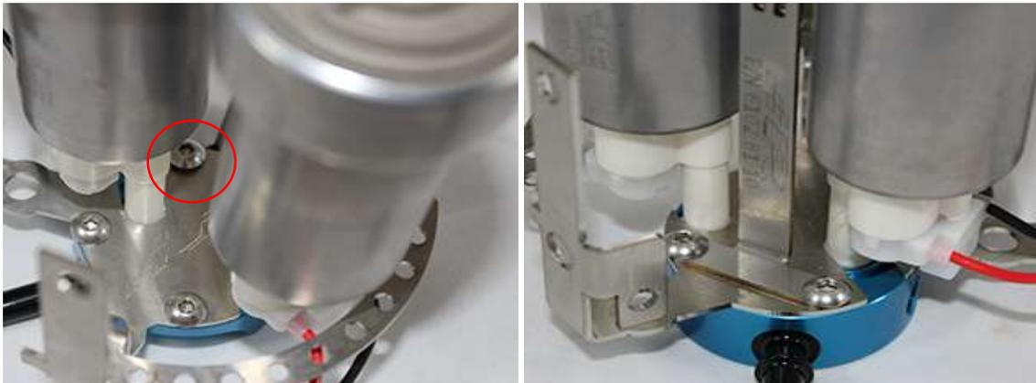
10. Insert the two supplied nylon zipties through the fuel support as shown below. Then secure both pumps to the fuel support with the zip ties, tighten, and cut off the excess.
