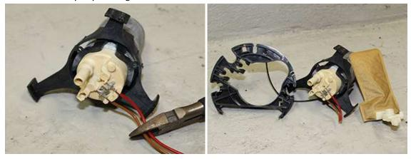
8. For this step you will take the bracket provided and install it as shown in the first image. The long tabs can be bent outward slightly if needed with a pair of pliers to help them better catch on the top of the bucket but is not required. Once it is sitting in place use a flashlight from the inside to make the holes for the bracket stand out then use a drill and <u>small</u> drill bit to mark the center of the hole on the outside of the bucket.
