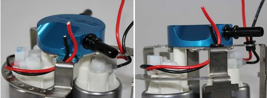
12. Now to install the pump assembly in the bucket by tilting the pump closest to the fuel float mount locations and as shown in the photo below. While doing this grab the bucket as seen in the other photo and squeeze slightly. For these photos we did not even touch the assembly only squeezed slightly on bucket for it to drop in so force is not required.
