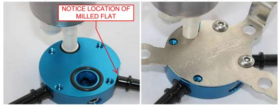
18. The pump will now be supported by the bracket but it needs to be treated with care for now. Install the 3<sup>rd</sup> screw as shown by only screwing in a couple threads. Once it is in slide the pump support bracket under the screw and install the 4<sup>th</sup> screw. Complete tightening of all 4 screws using a 3mm allen wrench.
