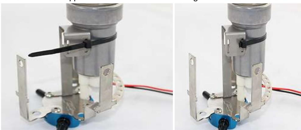
20. Cut the plug off the pump if it has not already been done. Insert the Red and Black wires through the hole located on the large bracket as shown in the image below. Then push the two wires through the supplied nylon grommet. Once the wires are through the grommet snap the nylon grommet into place on the bracket to ensure the wires are protected from any sharp edges. Finish this step by stripping and installing the supplied butt connectors.
