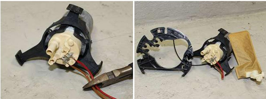
8. For this step you will take the bracket provided and install it as shown in the first image. The long tabs can be bent outward slightly if needed with a pair of pliers to help them better catch on the top of the bucket but is not required. Once it is sitting in place use a flashlight from the inside to make the holes for the bracket stand out then use a drill and small drill bit to mark the center of the hole on the outside of the bucket.
