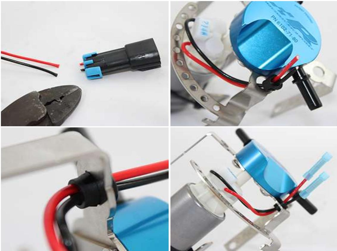
21. Take the factory plug with wires cut in step 7 of these instructions stripping both ends and crimping the supplied nylon crimp butt splice connectors to them. Then connect the Brown wire from the plug to the Black wire on the pump and crimp and repeat this step for the two Red wires.
