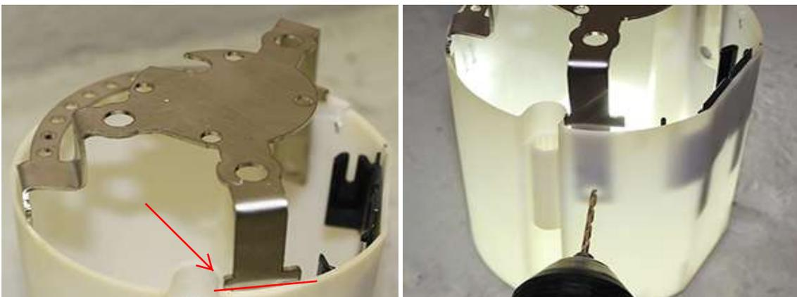
9. Once all 3 holes are marked on the outside of the bucket finish drilling through with the small bit working up to the final size bit which is 7/64". If you go from small to large instantly you risk cracking the bucket you do not have to use every size between the two but we advise at least 2 bits of in-between size.
