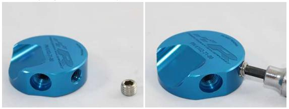
14. Take the blue manifold with the stainless plug inserted and two fittings supplied in your Precision Raceworks Stage 2+ Fuel Kit. Screw both fittings into the other two holes on the OD of the part. The fittings come with Oring seals preinstalled. Once the O-ring makes contact with the hole in the manifold they might need some pushing inward to continue going into the fitting.
