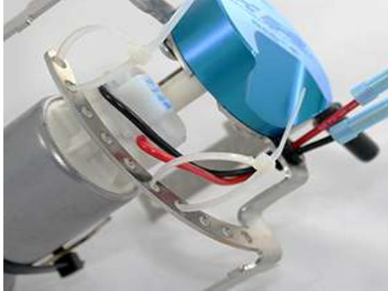
23. Install the supplied fuel sock onto the bottom of your Walbro 450 fuel pump tapping gently on the bottom of the sock below the port to insure it is completely seated on the pump.
