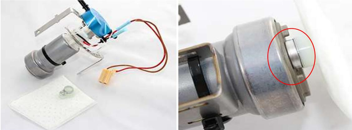
24. Insert the assembled Stage 2+ Precision Raceworks Fuel Kit into the bucket. You can remove the protective cap from the venturi fitting and push the venturi line onto the fitting while doing this to make it easier to do later. Align each of the 3 holes and using the supplied nylon push rivets secure the mounting bracket with assembly to the stock fuel bucket. Once the assembly is mounted reinstall the fuel float at this time
